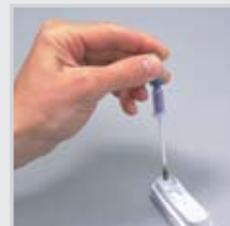
**3.** Squeeze the bulb to dispense 5 drops into the sample well.
