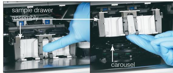
5. Remove the carousel by lifting up.
